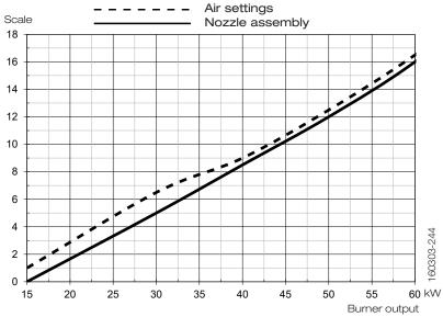
Scale value valid at 0 mbar in furnace pressure.
