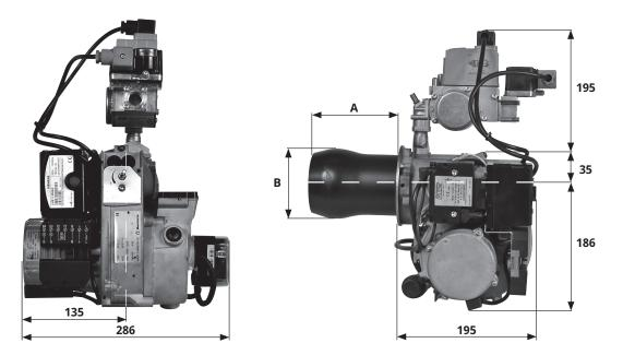
The above-mentioned measurements are maximum measurements. They can vary, depending on which components are used.
