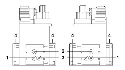
Screw plugs 1,2,3 may also be replaced by a measuring socket G 1/8 DIN ISO 228.
