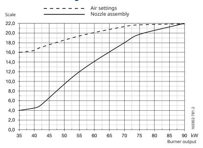
Scale value applies to 0 mbar furnace pressure.
