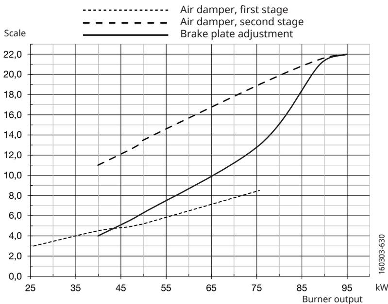
**!** Scale value valid at 0 mbar in furnace pressure.
