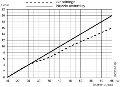
Scale value valid at 0 mbar in furnace pressure.
