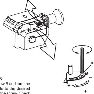
Loosen the stop screw B and turn the knob along the scale to the desired position and tighten the screw. Check the air adjustment by making a flue gas analysis.
